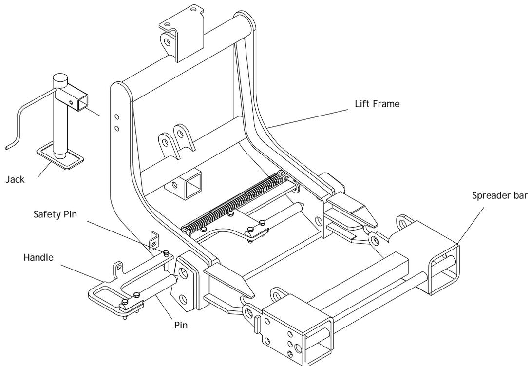
**NOTE:** Low mount lift frame is shown in picture. For removal of Quik link III HI DLC follow same procedure.
