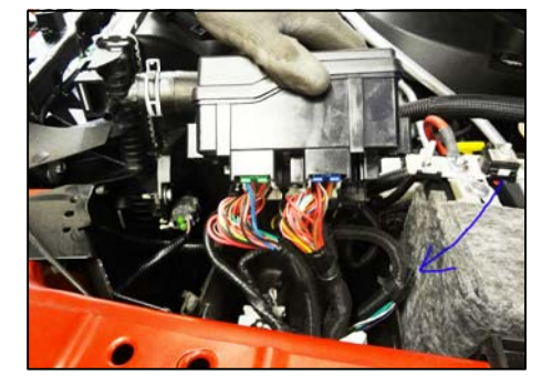
-lift the box and find 6 wires, attach them to the harness as shown
